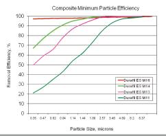
The above chart shows relative efficiency values at various particle sizes when tested in accordance with ASHRAE Standard 52.2-2007. When tested in accordance with Appendix J of that Standard the Durafil ES maintains these efficiency values throughout the life of the filter.
