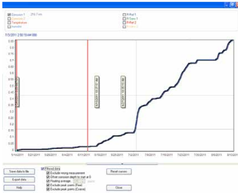
Fig. 3.1(b): Measured corrosion depth data, shown filtered.
