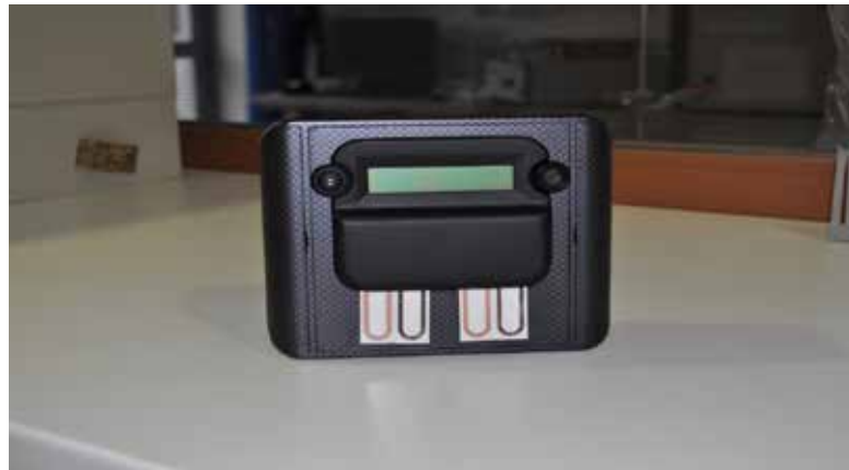
Fig. 2.1: Recommended positioning for the ISA-CHECK II logger
