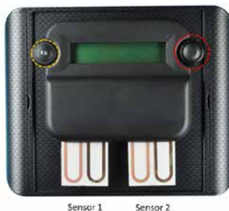
Fig. 1.2: ISA-CHECK II logger with two sensors. Red circle: push button activating the LCD screen, Yellow circle: control lamp (3 color LED).
