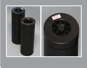
Adsorbent cylinders (available in two sizes) install on frames with a twist, and create tight filter-to-frame seal. A tool is provided that tightens the cylinder to the frame and ensues an air tight seal (see Product Sheet 2112 for cylinder information).
