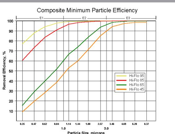
The above chart shows relative efficiency values at various particle sizes when tested in accordance with ASHRAE Standard 52.2-2007. When tested in accordance with Appendix J of that Standard the Hi-Flo maintains these efficiency values throughout the life of the filter.
