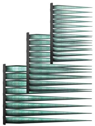
Hi-Flo ES air filters have a very long contaminant loading curve. Camfil Farr recommends ordering replacement filters when initial pressure drop doubles. This ensures that the required energy to move air through the filter is minimized.
