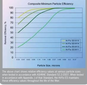
Air filters are the first line of defense to protect people and processes in buildings. The Hi-Flo ES can remove contaminants including fumes, smoke, bacteria, fungi, and virus-bearing droplet nuclei. The Hi-Flo ES is also the filter of choice for the removal of nuisance contaminants such as pollen, paper dust, and other atmospheric impurities.
