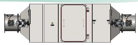
Typically dampers are installed upstream and downstream of the air filters that need to be serviced.
