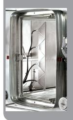
The internal scanning probe of Camfil CamContain equipment is controlled by the Motion Control Lite, precluding the human errors inherent to manual scanning. The four scanning modules of the CamContain are shown in the photo (left).
