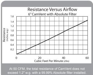
The Camfil CamContain CamVent is a slim and compact HEPA filter system. It is ideal for filtering plumbing vent stacks or as a HEPA filtered tank displacement device. It is well suited as a secondary HEPA filter system for biosafety cabinets. It may be used as a transfer HEPA filtering system to accommodate system pressure pulses between two biosafety zones. The Camfil CamContain CamVent:
