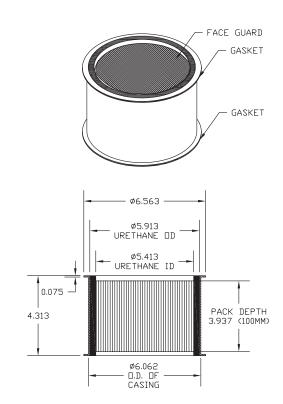
Non-Intrusive Filter Validation Biocontainment Venting System
