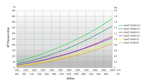
Camfil filters are tested in our R&D center in Trosa, Sweden and also at a third party, in accordance with EN779 and ASHRAE 52.2. In addition burst pressure tests have been conducted according to the industry's latest and most stringent standards.
