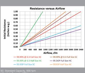
The Camfil Absolute VG provides high-efficiency particulate air (HEPA) filtration for critical application processes. Its critical media mass, is more than twice that of standard HEPA filters, which ensures low resistance to airflow for optimal energy savings throughout the life of the filter and increased air changes for air-starved applications. The Camfil Absolute VG filter offers:
